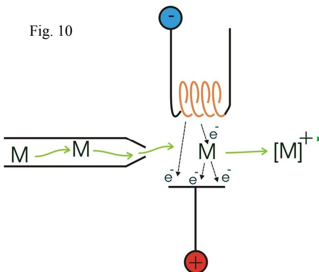
The process of ionization involves a high-speed electron (70eV) colliding with a gas molecule. It adds enough energy for one of the molecule's own electrons to escape, leading to a positive, free-radical ion.
