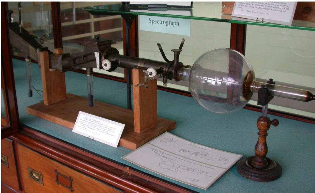
Fig. 9 – Aston's third mass spec tube; obviously the magnets etc. are not included
