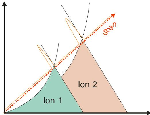
Fig. 13 – scanning a quadrupole
