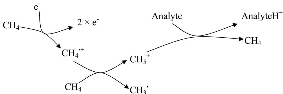
Fig. 17 – charge transfer mechanism for methane as ionizing gas in CI. Note that not all ions become positively charged this way. It is also possible for  $CH_5^+$  to remove a complete neutral hydrogen from something resulting in  $CH_4$ ,  $H_2$ , and  $Analyte^{\cdot}$ .
